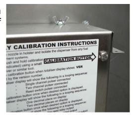
Gently push and hold the calibration button using a small screwdriver or similar tool.
